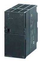
SIPLUS S7-300 PS 307 based on 6ES7307-1EA01-0AA0 with conformal coating, -  $25...+70~^\circ\text{C}$  , stabilized power supply input: 120/230 V AC output: 24 V DC/5 A
