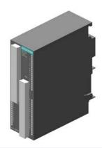
SIMATIC S7-300 digital output SM 322, Isolated in groups of 16, 64DO, 24 V DC, 0.3A sink output Total current 2 A/group, 8 A/module Terminal blocks 6ES7392-1.N00-0AA0 and cable 6ES7392-4...0-0AA0 required
