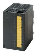
$^{\star\star\star}$  Spare part  $^{\star\star\star}$  SIMATIC S7, Digital output SM 326, 10 DO, 24 V DC, 2A, fail-safe digital output for SIMATIC S7F systems, with diagnostic alarm, 1x 40-pole
