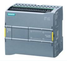
SIMATIC S7-1200F, CPU 1214 FC, compact CPU, DC/DC/relay, onboard I/O: 14 DI 24 V DC; 10 DO relay 2 A; 2 AI 0-10 V DC, Power supply: DC 20.4-28.8V DC, Program/data memory 125 KB
