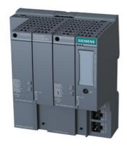
XF201-3P IRT managed IE IRT switch, 1x 10/100 Mbit/s RJ45 ports, 3x 100 Mbit/s POF SC RJ Ports, Bus adapter assembled, Error signaling contact with set pushbutton, redundant power supply, PROFINET IO device, network management, Redundancy Manager integrated, incl. electron. manual on CD-ROM, C-PLUG optional.
