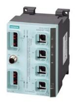
SCALANCE X204IRT PRO, managed IE IRT switch with degree of protection IP65/67, 4x 10/100 Mbps push-pull RJ45 ports, error signaling contact with set button; power supply (load/encoder); PROFINET IO device, network management, Redundancy Manager integrated, incl. electron. manual on CD-ROM, C-PLUG optional.
